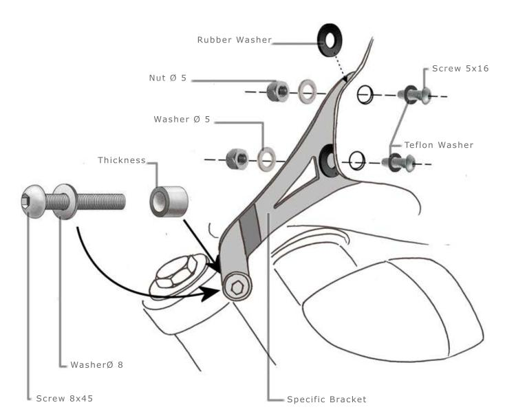
PUT THE TWO BRACKET ON THE STEERING PLATE, LIKE DESCRIBED IN THE PICTURE. ONCE YOU MOUNTED THE BRACKET, WITHOUT LOCK, MOUNT THE PLEXIGLASS ON IT, PUTTING THE SCEWS AND THE WASHERS FOLLOWING THE PROCEDURE DESCRIBED IN THE PICTURE.FIND THE IDEAL POSITION OF WINDSHIELD/SCREEN AND THAN LOCK ALL. DON'T LOCK TOO MUCH THE SCREW 5X16 ON THE PLEXI-GLASS TO AVOID DAMAGES.
